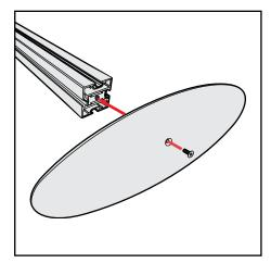
Base Plate & Extrusion Connection
